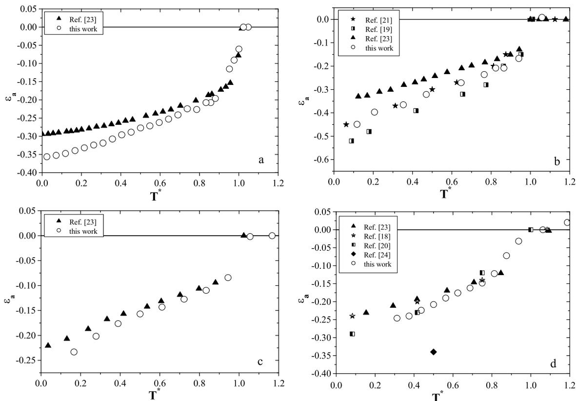
**Figure 1: The dielectric anisotropy  $\epsilon_a = \epsilon_{\parallel} - \epsilon_{\perp}$  of 5/8 (a), 8/7 (b), 10/4 (c) and 10/6 (d) as a function of the relative temperature  $T^* = (T - T_N)/(T_{NI} - T_N)$ , where  $T_{NI}$  is the clearing point and  $T_N$  is the lower temperature limit of the nematic range.**
