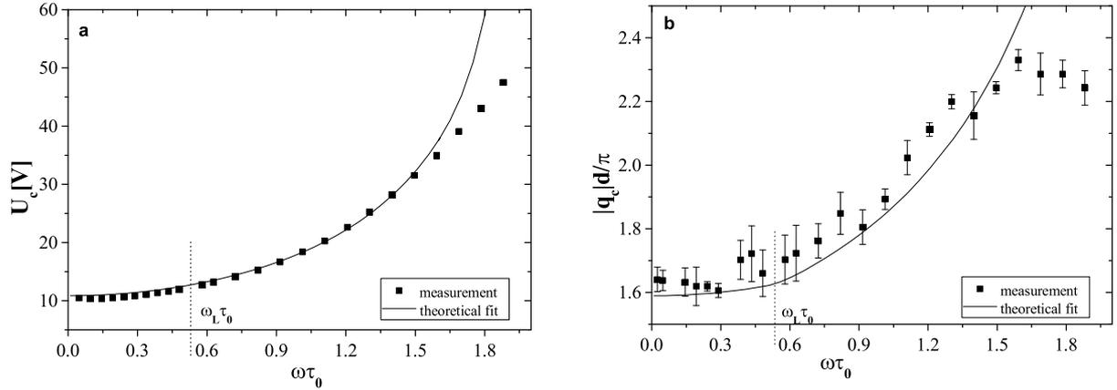
**Figure 6: Comparison of the measured data (squares) and the theoretical predictions (solid line) for the dependence of the threshold voltage  $U_c$  (a) and the critical wavenumber  $|q_c| = \sqrt{q_x^2 + q_y^2}$  (b) on  $\omega\tau_0$ , for 10/6 at  $88^\circ\text{C}$  ( $T^* = 0.8$ ). The dotted line denotes the Lifshitz point.**
