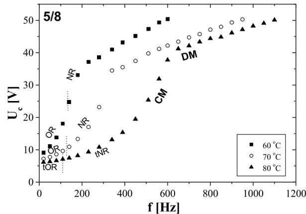
**Figure 3:** The EC threshold voltage  $U_c$  for 5/8 as a function of the frequency  $f$  at three different temperatures. CM, DM, NR, OR, tNR and tOR denote the conductive mode, the dielectric mode, normal rolls, oblique rolls, travelling normal rolls and travelling oblique rolls, respectively. The vertical dotted lines denote the Lifshitz points.
