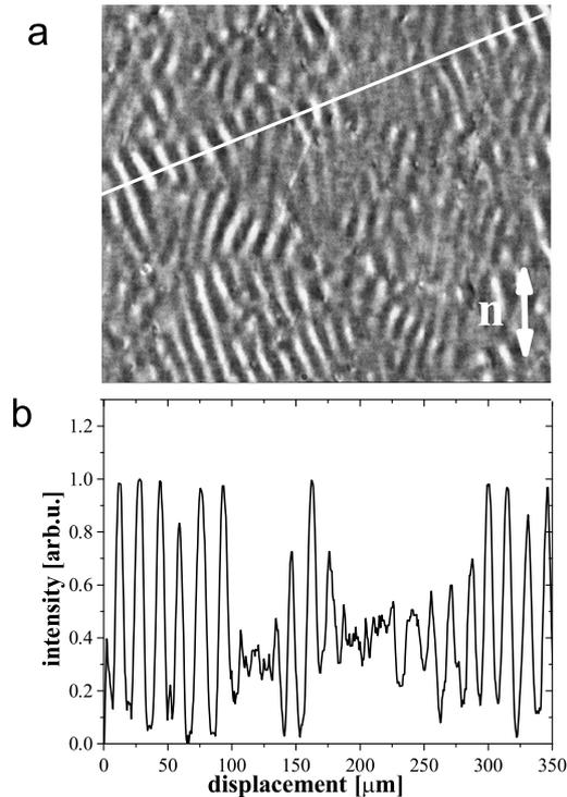
**Figure 7:** Snapshot of the ns-EC structure (oblique stripes, OS, see the text for description) taken with crossed polarizers (a) and the corresponding intensity profile (b) along the white line for 10/6 at  $T = 85^{\circ}\text{C}$  ( $T^* = 0.4$ ),  $f = 100\text{Hz}$  ( $\omega\tau_0 = 0.42$ ) and  $\varepsilon = 0.32$ . The director is vertical as it is shown by the white arrow and it is parallel to one of the crossed polarizers.
