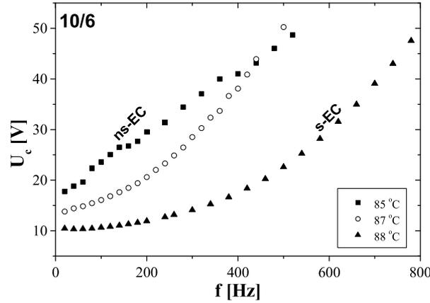
**Figure 8:** Threshold voltage  $U_c$  versus frequency  $f$  of the structures observed in 10/6 at three different temperatures.
