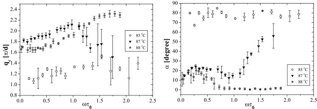
**Figure 9:** The dependence of the critical wavenumber  $|q_c| = \sqrt{q_x^2 + q_y^2}$  and the obliqueness  $\alpha = \arctan(\frac{q_x}{q_y})$  on  $\omega\tau_0$  for 10/6 at  $85^\circ\text{C}$  ( $T^* = 0.4$ ),  $87^\circ\text{C}$  ( $T^* = 0.66$ ) and  $88^\circ\text{C}$  ( $T^* = 0.8$ ).
