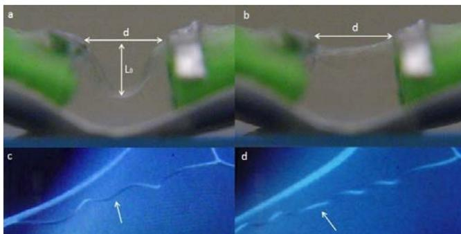
Figure 1 – Cellulose liquid crystalline electrospun materials. (a) and (b) represent the spontaneously changing membrane shape and size modification, (b) was recorded 175 min after (a);  $d = 4$  mm. (c) and (d) Scanning electron microscopy (SEM) images; evolution of a microhelical structure. Electron beam irradiation at the arrow-pointed spot (photo (d) was taken 16 s after photo (c))
